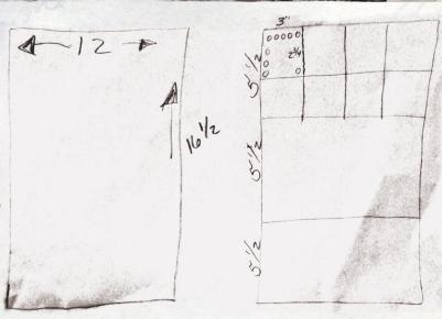
The clutch then folds into (3) five and a half inch sections (front, back, and lid) The side gusset(s) were made out of pieces that were cut to five and a half inches tall by two and three-quarters. Fold in half lengthwise and stitch from corner to one inch mark on the fold.
